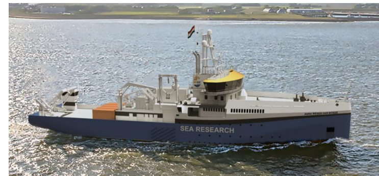
79 m RESEARCH VESSEL (GAS-OIL METHANOL DUAL FUEL+ batteries)
