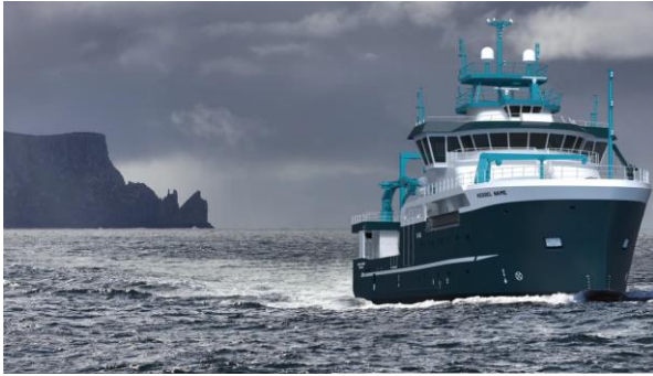
56 m RESEARCH VESSEL (DC GRID+ BATTERIES)
